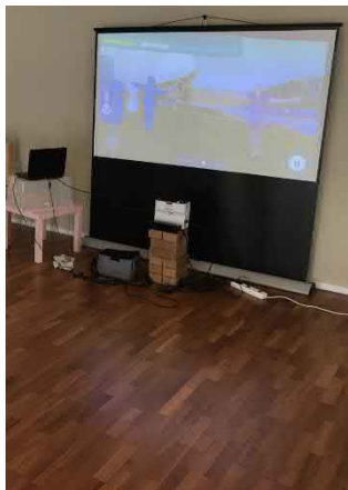
Figure 4: The hardware setup was consistent between both versions. Users faced a 240x135cm screen driven by an ultra-short distance projector. A Microsoft Kinect V2 tracked the users.
